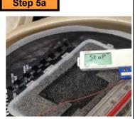
Remove the data logger from the box. You can now follow the Data Station instruction to download temperature data, if needed
