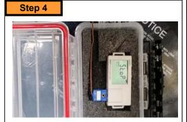
Open the Data Logger Box. If you are not downloading data, Go to Step 5a. If your Data Station Software is installed on a nearby computer, Go to Step 5a. Otherwise Go to Step 5b.
