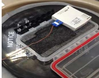
Remove the data logger from the box. You can now follow the Data Station instruction to download temperature.
