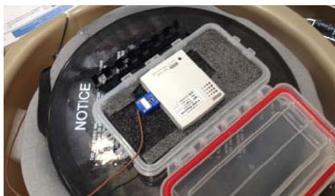
Open the Data Logger Box. If your Data Station Software is installed on a nearby computer, Go to Step 5a. Otherwise Go to Step 5b.
