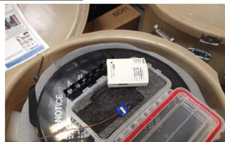
If your Data Station Software is not installed on a nearby computer, disconnect Thermocouple from Data Logger. You can now follow the Data Station instruction to download temperature data.
