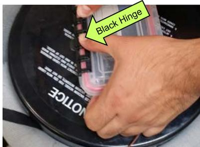
Unlatch Data Logger box using thumbs to press against the black hinge.
