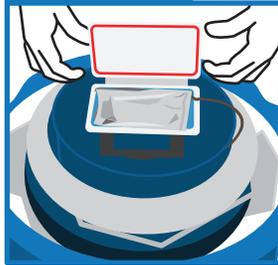
Open the lid and expose the data logger in its metalized pouch.
