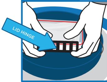
Unlatch data logger using thumbs to press against the black hinge.
