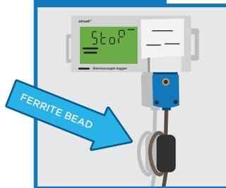
Follow the Data Station instructions to download temperature data, if desired. The data logger may be detached from the thermocouple to move to a remote computer to download data. Once completed go to Step 5b.
