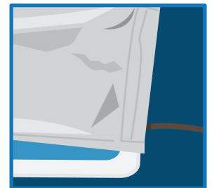
Place data logger back into the pouch and make sure to push the cable with the ferrite bead completely down into the bag. Push the cable into the far corner of the bag and reseal by pushing all the way across the zip lock seal.
