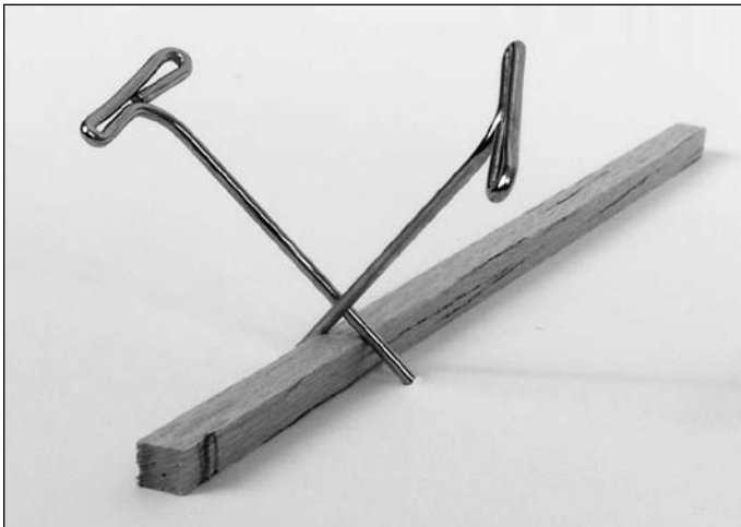
Figure 26 – Cross two pins over the piece of wood to hold it in place.
