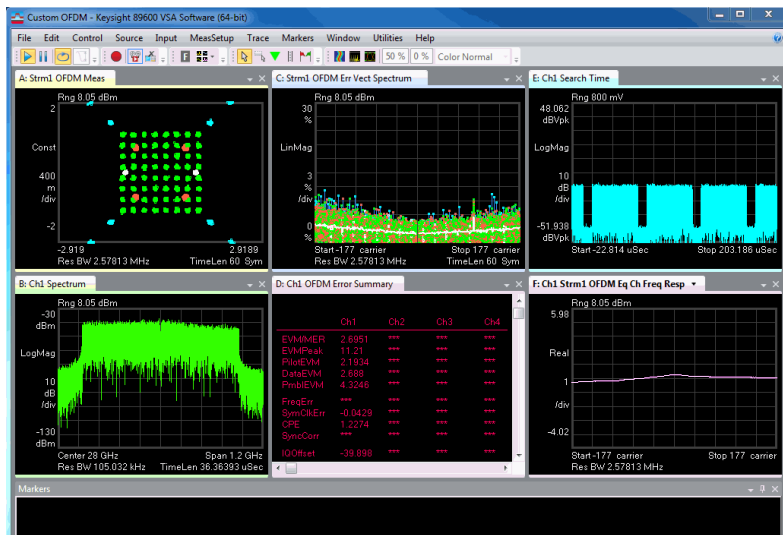
Figure 17. This display from the 89600 VSA software provides multiple views of the demodulated OFDM signal.
