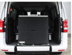
The tailgate can be closed with the access ramp in a vertical position, leaving sufficient space for an empty wheelchair or other cargo.
