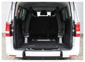
With seats stowed, the Metris WAV ramp can be folded down to create a level floor for additional storage space.
