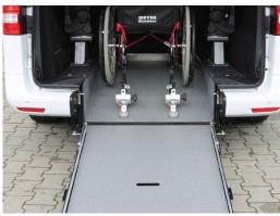
The Metris WAV comes equipped with an automatic tensioning system that assists with loading and unloading a wheelchair passenger. Rear securement retractors provide an efficient, easy-to-use, 4-point tie-down system.
