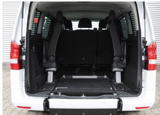
With seats stowed, the Metris WAV ramp can be folded down to create a level floor for additional storage space.
