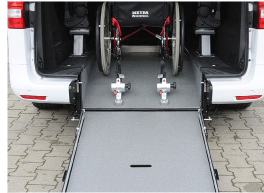
The Metris WAV comes equipped with an automatic tensioning system that assists with loading and unloading a wheelchair passenger. Rear securement retractors provide an efficient, easy-to-use, 4-point tie-down system.
