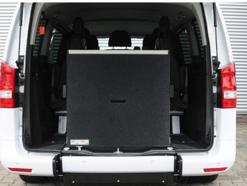
The tailgate can be closed with the access ramp in a vertical position, leaving sufficient space for an empty wheelchair or other cargo.
