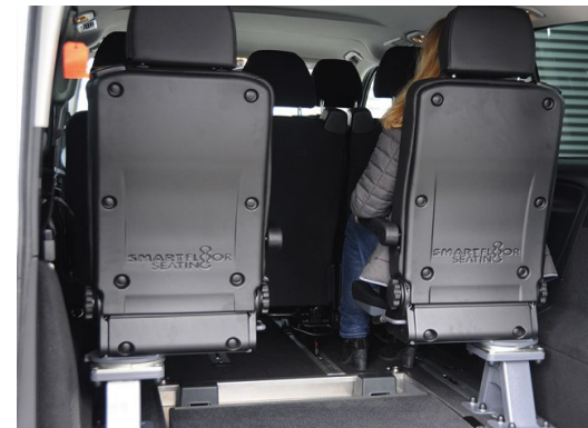
With the access ramp fully folded away and the rear seats in their original position, the vehicle can be used as a standard vehicle.
