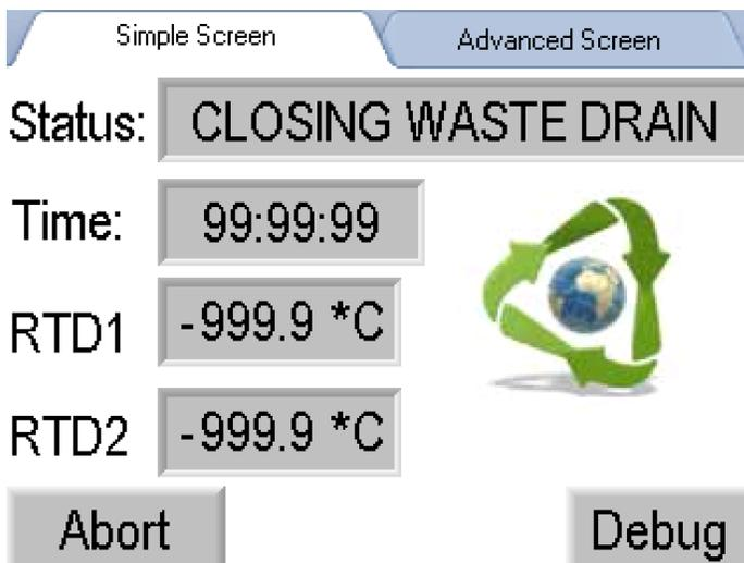
After the tank drain timer times out, the recycler will automatically advance to the this display that will alert the user that the waste drain is now closing. The recycler will attempt to close the waste drain for 10 seconds. Once the drain has been closed, the recycler will automatically advance to the next stage. All buttons function as previously stated.
