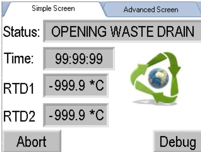
The next stage of the recycling process is the tank drain. This is the screen that the user will see during the drain open process.. All buttons function as previously stated.
