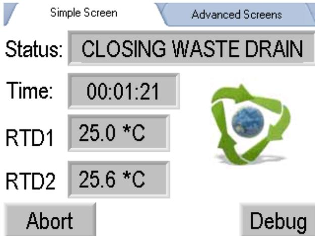
When the draining time has ended the waste drain will close.
