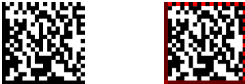
Figure 2—Typical Data Matrix Code
