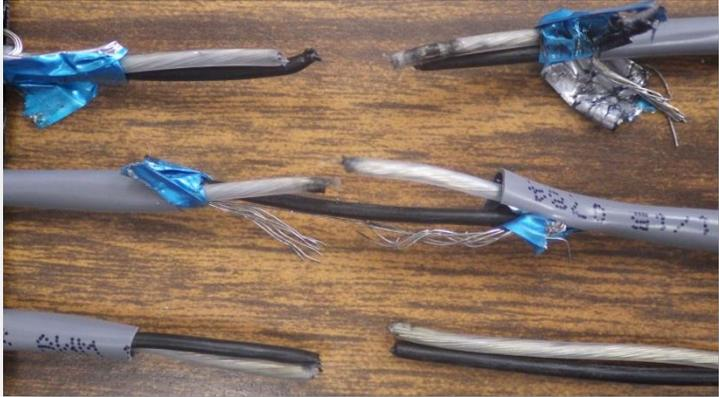
Competitor cables after failing in flex test. Belden retains circuit 2.8 times longer
