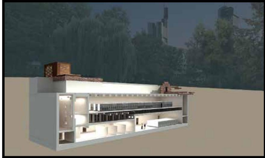
The new substation approach: small surface footprint with levels underground
