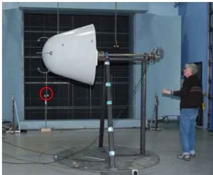
Figure 3 Concept tests in a 4x4 m 2 wind tunnel. The spinner is yawed to -90° and the "classic" sonic sensors can be seen on the nose. The cup anemometer is seen in the lower left corner of the inlet (encircled).
