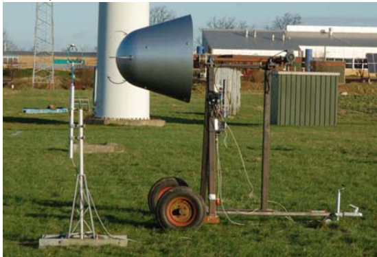
Figure 11 Arrangement of the S300 spinner anemometer with "new" sensors in comparison with the sonic anemometer at Risø test site
