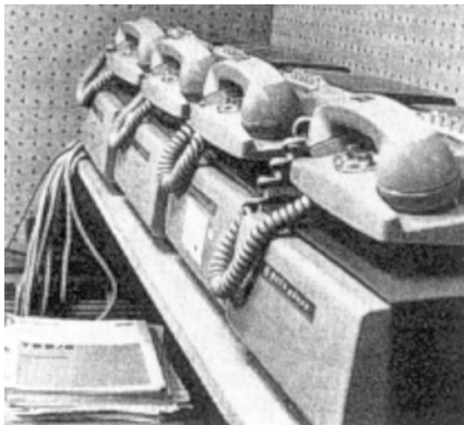
The Dataphone, the first commercial modem, designed by Bell Labs
