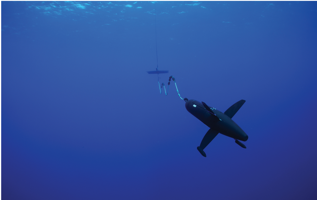
Figure 2 - Liquid Robotics towbody and motion isolating cable
