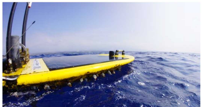
Fig 3 – Biofouling on the sides and bottom of the float
