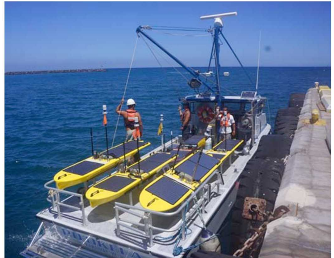
Fig 6 - Deploying multiple Wave Gliders on a single vessel
