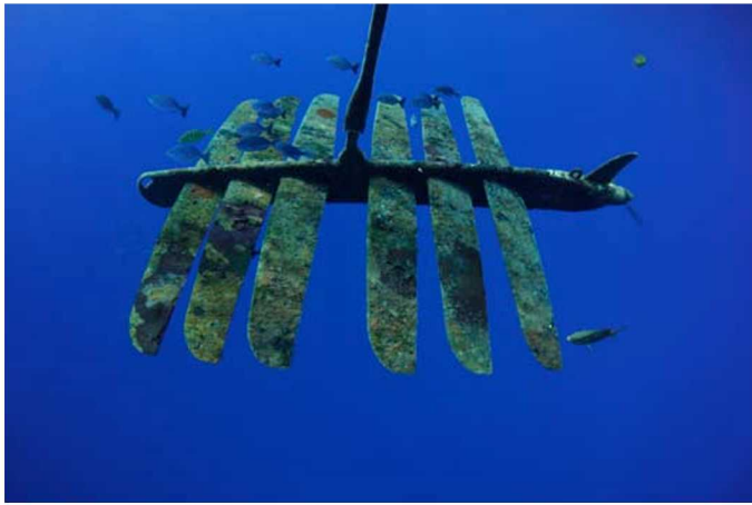
Fig 4 - Biofouling on the sub and wings
