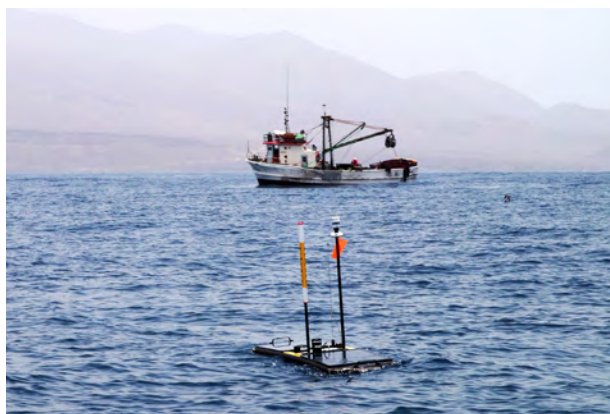
The Wave Glider measuring CO 2 and O 2 exchange at the air/sea boundary in the Cape Verde Archipelago. Image courtesy of GEOMAR.
