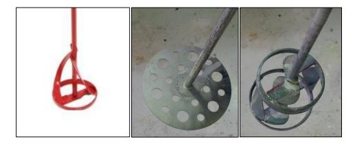
For smaller volumes a stirrer along the lines of the below image must be used so that the RPM can be achieved without the paint splashing out of the drum.
