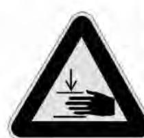
**When replacing blades, stop the air supply or disconnect the air hose.**
