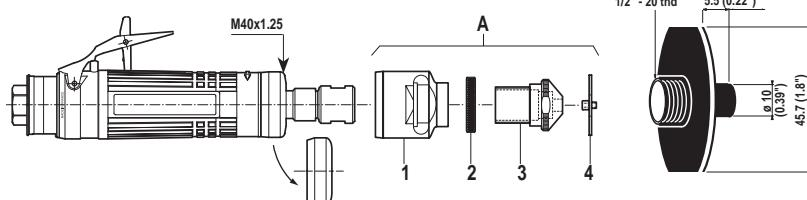
615 396 289 0: Machined routing kit for burr, max ø 6.4mm (1/4")
