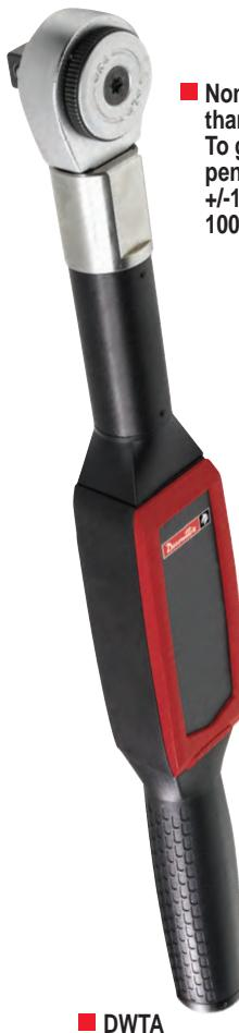
■ Non Length Dependent Transducer thanks to double bridge strain gauge. To guarantee a tightening result independent from operator hand position +/- 1 % of torque reading (from 10 % to 100 % of torque range)
