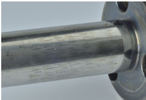
Normal wear, short stroke (example: guide plates)
