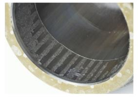
Normal wear pattern. Depending on the load capacity, the contact pattern is approximately 120° with a circular sector – for low requirements, the fine centering bushing can be rotated twice by 120° in relation to the pillar/cage in order to extend the lifespan.
