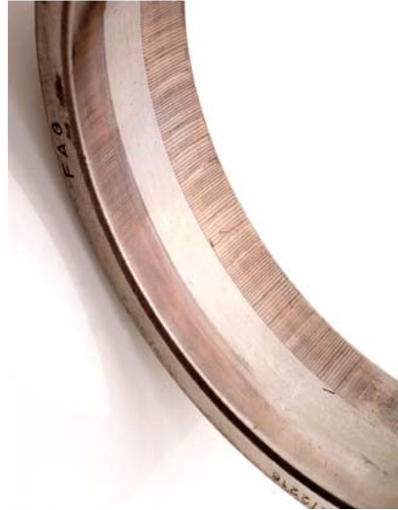
Current Fluting Damage
