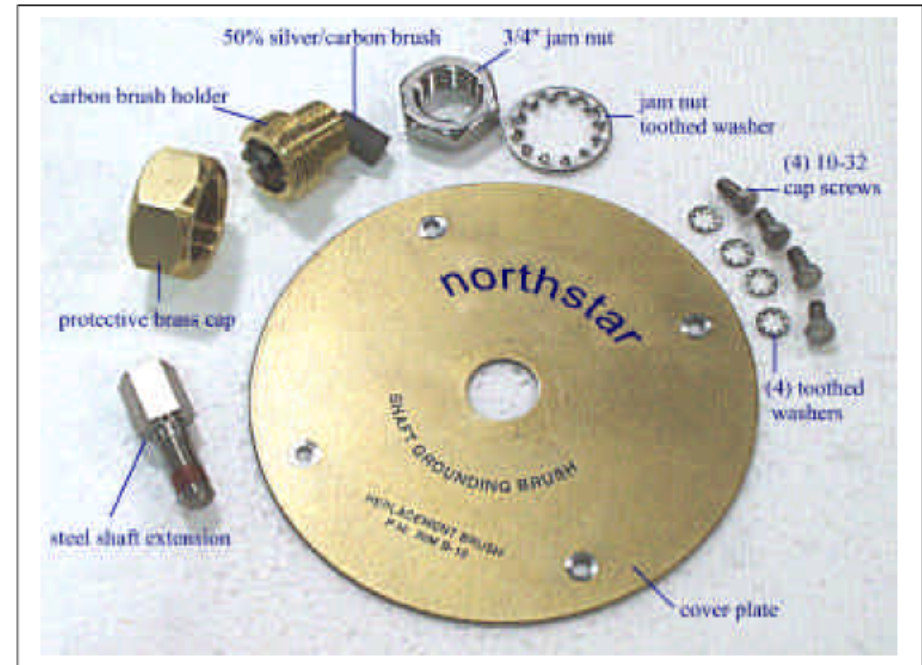
Figure 3: Components of RIM Tach ® Shaft Grounding Brush Assembly (end-of-shaft)
