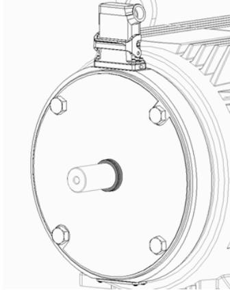
**9.0** Remove matting connector from unit, unscrew (4) mating connector screws.
