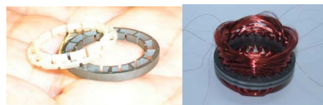
Figure 6: The stator coil of the resolver consists of the lamination (metal, left) wound with wire in a variable pattern (right). The white ring on the left is an end insulator.
