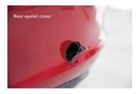
Press bottom of rear eyelet cover to remove.
