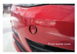
Press left side of front eyelet cover to remove.
