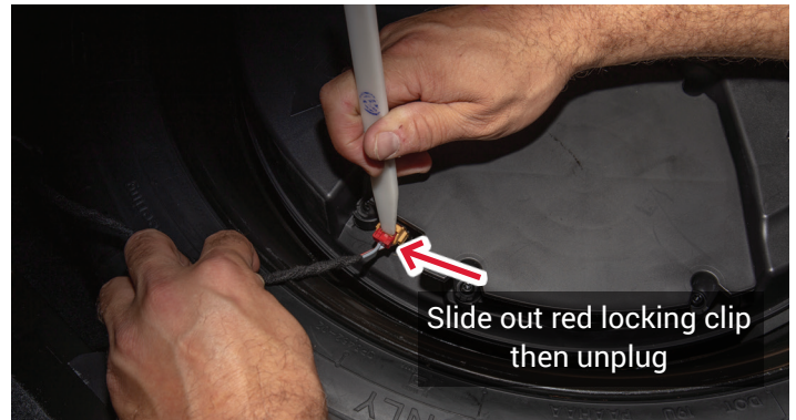
Unplug the subwoofer, and spin off the retainer nut to remove.
