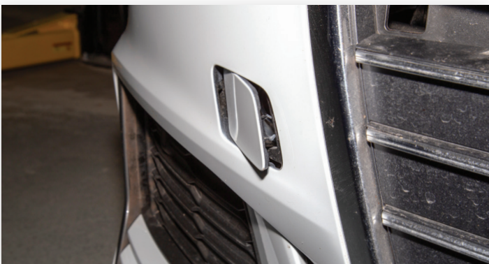
On the front bumper, press the left side of the front eyelet cover to remove.
