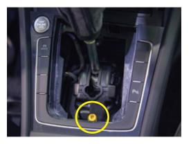
Pull the shift boot/bezel assembly over the shifter.
