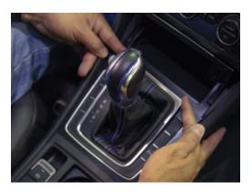
Open the coin tray in front of the shifter. Pull up on the front of the shift boot/ bezel assembly to release.
