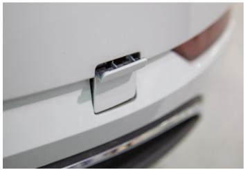
**REAR:** Press the bottom of the rear eyelet cover to remove.
