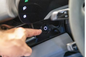
Leave the outside 12-volt source connected for at least 5 minutes or until the dash cluster illuminates when pressing the power button on dash.
