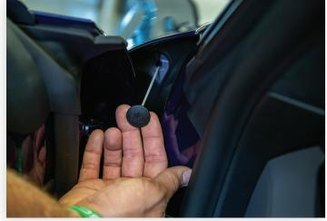
Pull the release towards the back of the vehicle. Remove the charge cord from the charge port.
