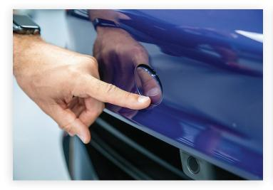
Front eyelet cover – press in at the bottom.
