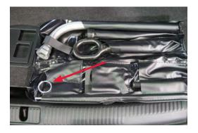
The OEM provided ring tool can be found with the vehicle's jack and tire tools.
