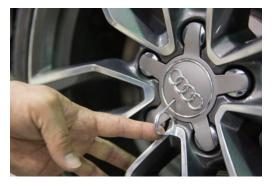
Engage "hook" on the tool's tip through the hole in the cover and gently pull straight out, removing the cover.
