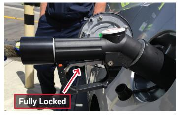
Lift lever fully to locked position.
