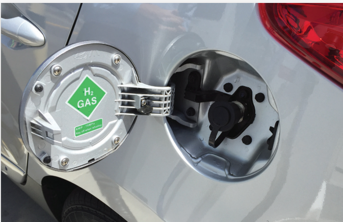
Green hydrogen gas decal and fitting in filler door
