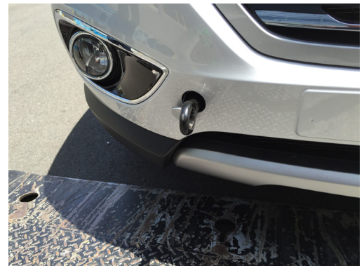
Tow Eyelet installed in Front Provision
