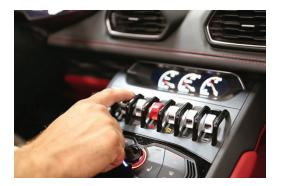
With the vehicle running, pull the nose lift switch down.
