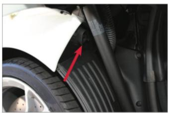
The Service Provider can access the front cargo area where the start battery is housed via the manual release found in the driver's side lower door opening. See arrows below.
