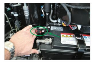
The CAN Plug MUST be reconnected before reassembly of the cargo area.
