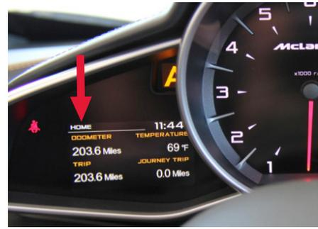
Move the control stalk upwards scrolling through the various selections to: Vehicle Info
