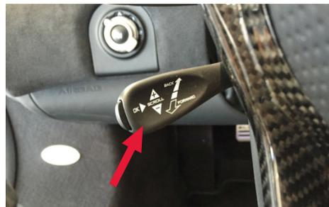
Prior to navigating the left hand display any error messages or reminders will first need to be acknowledged. These faults are stored and can be recalled at any time; acknowledgement does not mean they have been erased. On the left hand side of the steering column, below the turn signal stalk, is the control stalk for the left hand display.
