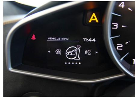
Once at the Vehicle Info menu scroll down to "Battery Status" and select by pulling the control stalk backwards.
