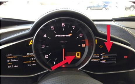
The elements that acknowledge the vehicle is in Ignition State 5:
