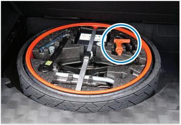
Retrieve orange Park Release handle in Tool Kit under load floor
