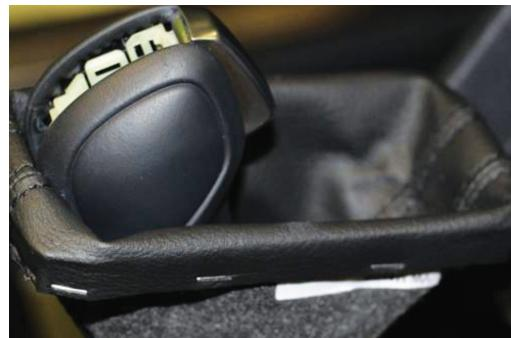
Carefully remove shifter boot from console.
