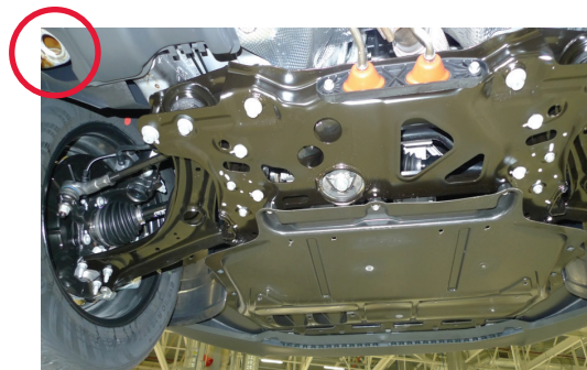
The NMS Passat has no tow eyelet provisions, front or rear.
