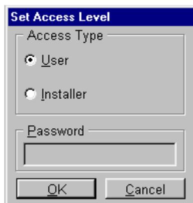
Click on the desired access type, enter the password, and click *OK*. If an incorrect password is entered, the software will automatically default to *USER* level.
