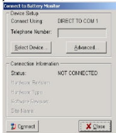
Click on the *SELECT DEVICE* button to select the appropriate device to use to connect to the *PowerShield* system. *PowerShield* systems can be set up to communicate via a direct serial link, a modem, or over an Ethernet LAN using TCP/IP.
