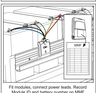
Fit modules, connect power leads. Record Module ID and battery number on MMF.
