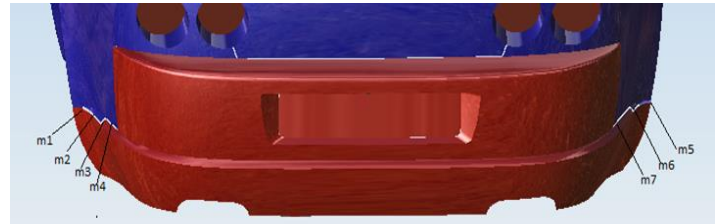
Figure 4. Measurement Points for Study. These seven locations are the measurements used to view the amount of variation from the gravity and thermal effects.
