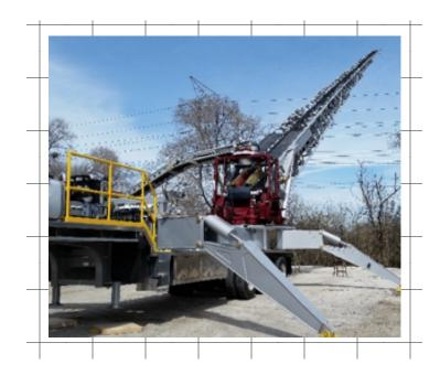
the surface. Loop Belt's conveyor systems seemed an obvious choice to help the fracking teams achieve their goals, but the switch from pouring concrete to delivering sand required redesigning some elements of the conveyor system.
