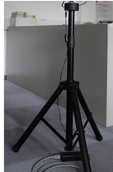
Figure 21: Rotary Tripod with motor slip ring for electrical transmission
