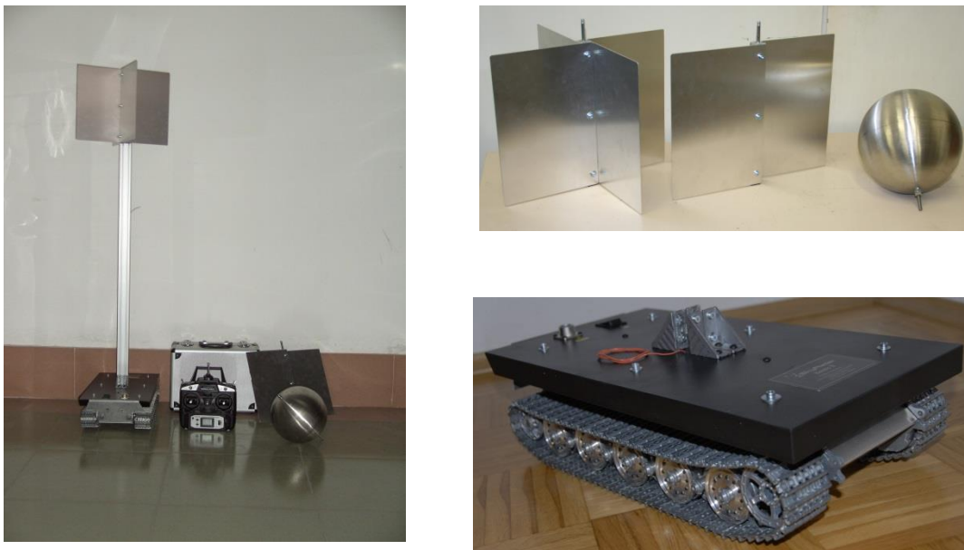
Figure 28: Remote controlled moveable target with 3 different reflectors.
