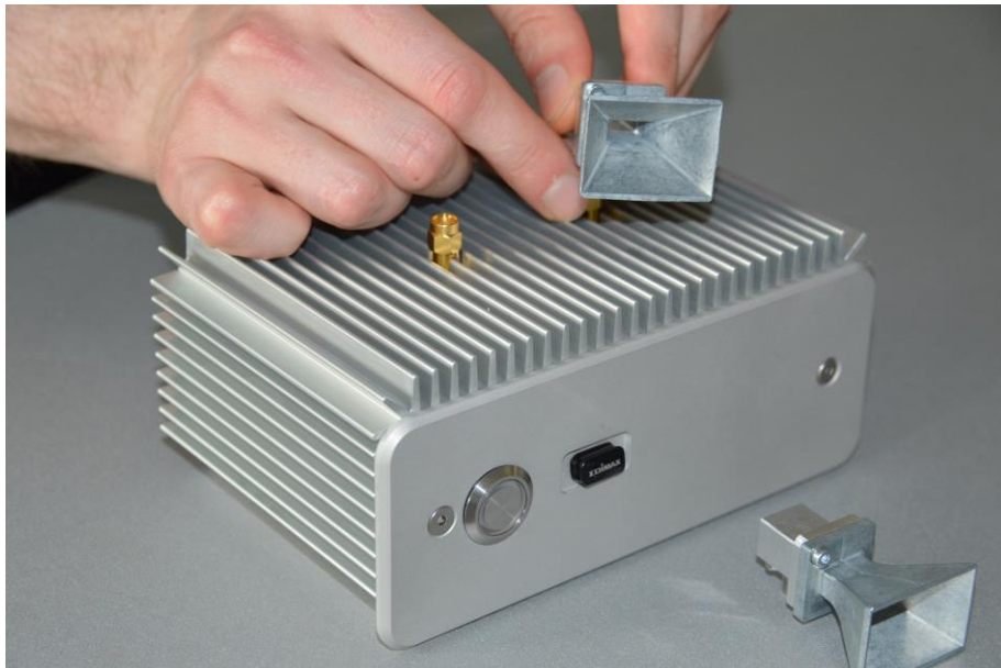
Figure 17: User exchanges an antenna plug and play in seconds
