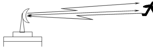
Fig. 1 The principle of operation of radar
