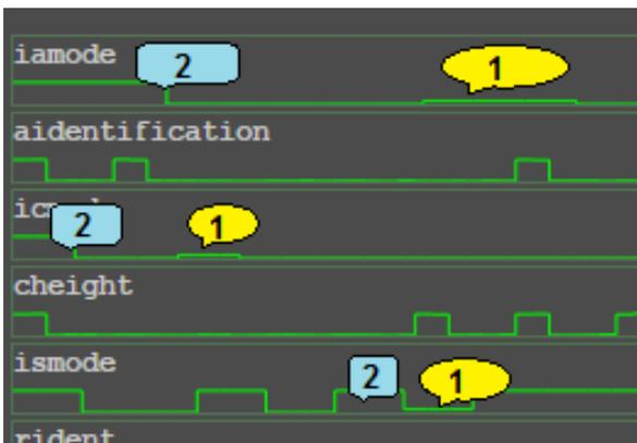
The signal (1) from omnidirectional antenna is less than signal from directed antenna (2). This means that the captured aircraft flies in the mainlobe of monopulse radar. Other segments of the signal originating from other aircrafts, which are not flying in the mainlobe will not be processed as long as the radar antenna isn't directed to them.
