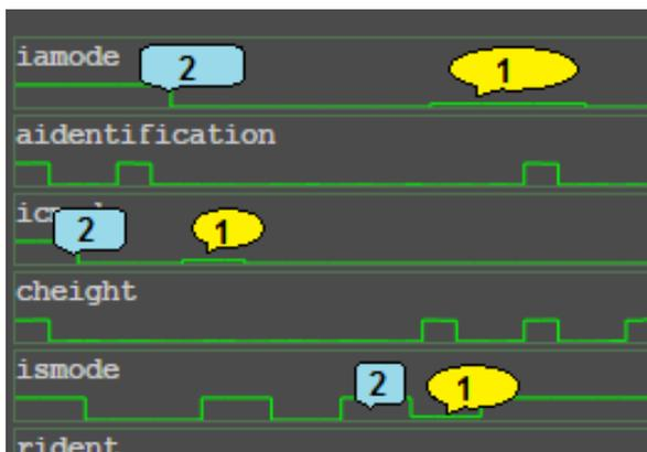
The signal (1) from the omnidirectional antenna is less than signal from directed antenna (2). This means that the captured aircraft flies in the main-lobe of the monopulse radar. Other segments of the signal originating from other aircrafts, which are not flying in the main-lobe, will not be processed as long as the radar antenna isn't directed to them.
