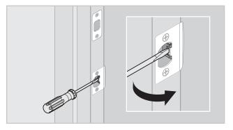
The lower latch and lower strike (for your knob or lever) are misaligned, putting too much load on the deadbolt latch.
