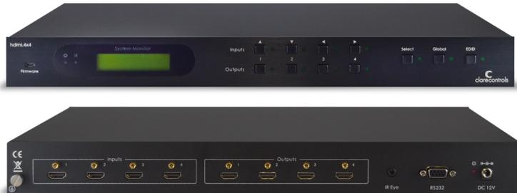
The Clare 4x4 HDMI matrix switcher enables independent crosspoint switching from any of four inputs to any or all of four output devices. Features include smart EDID management, ultra-fast switching, and support for 1080p and 3D. The HDMI 4x4 includes drivers for easy integration into Clare Controls, Crestron, Control4, Elan, and RTI control systems.
